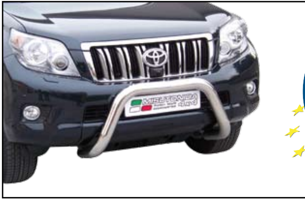
EC/SB/255/IX EC APPROVED Super Bar Ø 76 mm
