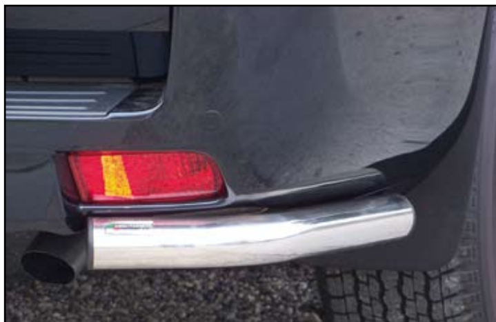
PPA/255/IX Angular Rear Protection Ø 63 mm
