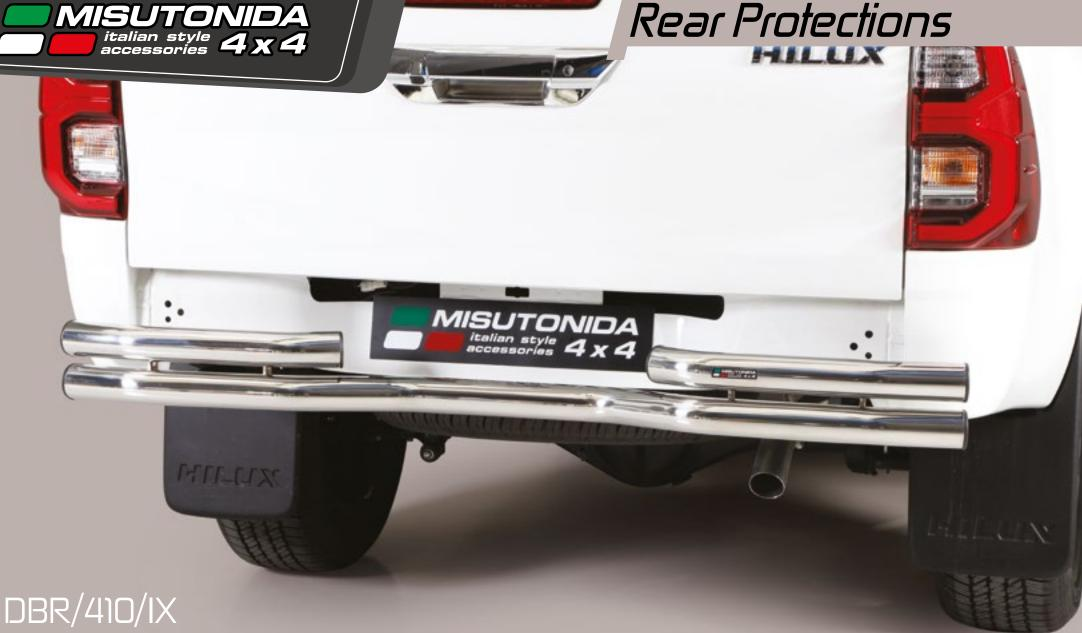
Double Bended Rear protection Ø 63mm. Also available in Black Powder Coated version DBR/410/PL
