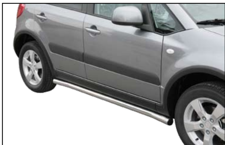
TPS/258/IX Side Protection Ø 63 mm
