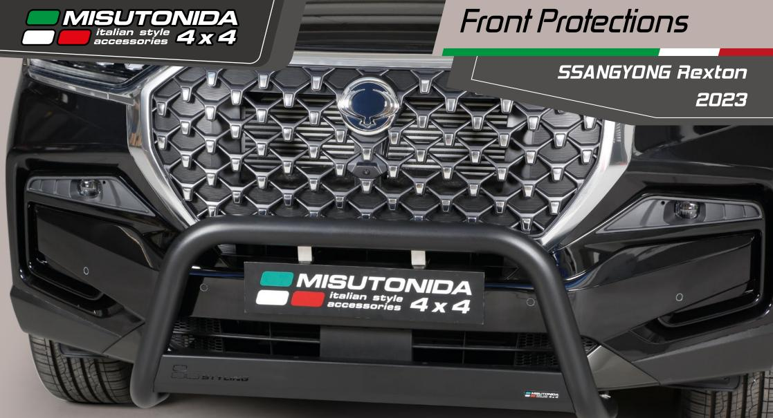
MED/435/PL Black Powder Coated Medium Bar Ø 63mm. Compatible with front camera, ACC System. In case of park sensors, use our park sensors stickers to fit the front guard.
