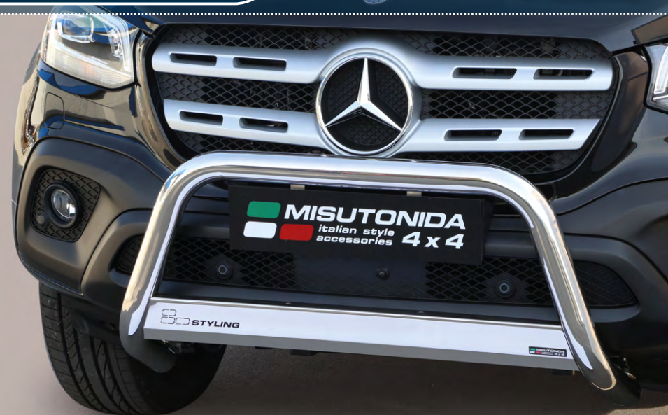
MED/428/IX* Medium Bar Ø 63mm / also available in Black Powder coated version MED/428/PL*
