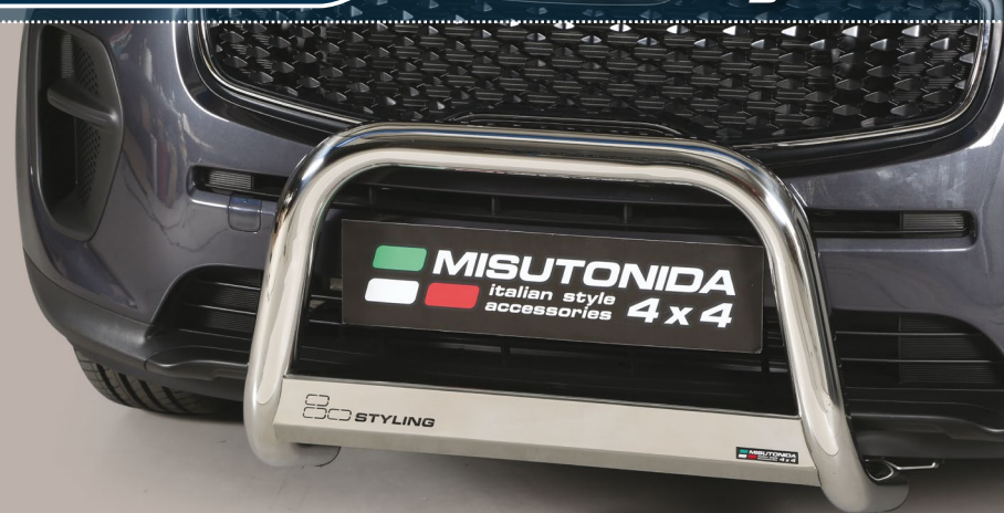
MED/403/IX* Medium Bar Ø 63mm also available with mark MED/K/403/IX*
